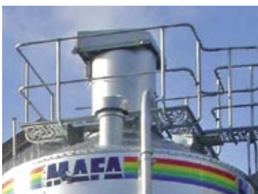
Platform, vertical ladder and filter.
